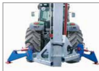
Hydraulically folding tower support feet for abetter stendness (Mammoth-Titan)
