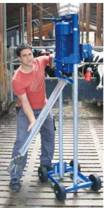
The **propeller blades** open through the centrifugal force as soon as the motor is switched on.
