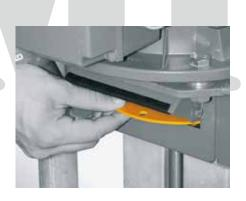
With the **turntable**, the propeller can be easily turned into the right position to get it out through the fissures.
