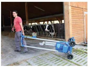
This is very practical during transport. An additional transport cart is not necessary. When folding up no slurry flows over the motor.
